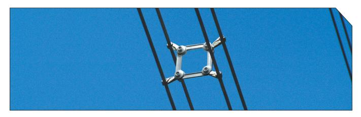
PLP's range of CUSHION-GRIP Spacer Dampers feature elostomer damping elements engineered to absorb maximum energy and protect valuable line hardware. The design provides utmost resistance to conductor fatigue and eliminates the need for additional Stockbridge type dampers. The CUSHION-GRIP range is available for twin, Tri, Quad and hex bundle configurations.
